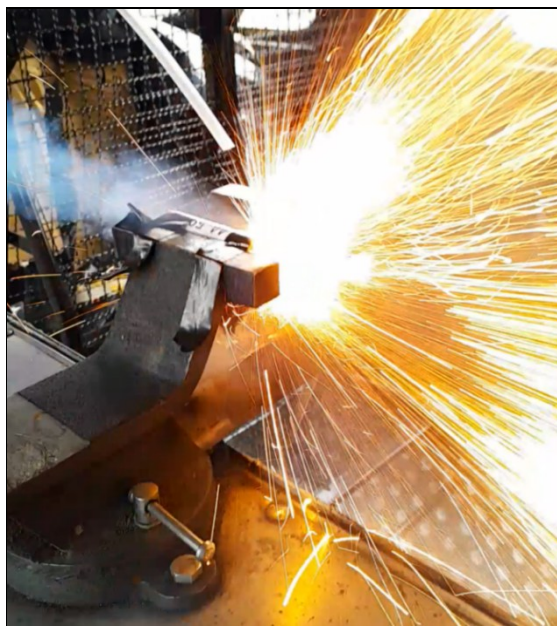
Fig. 2. Thermal runaway in an NMC 18650 cell during the nail puncture test
