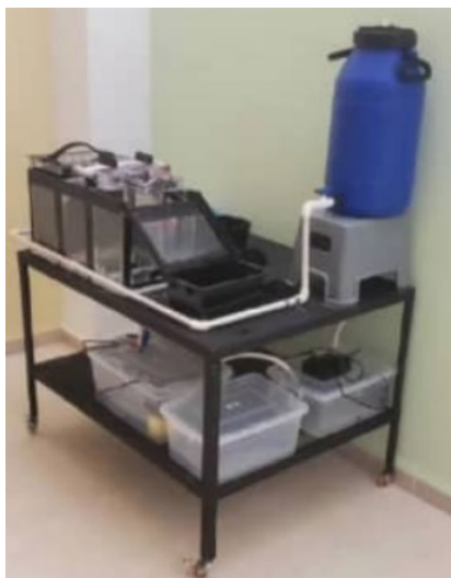
Fig. 4. Electrocoagulation treatment prototype using a conventional parallel-flow configuration
