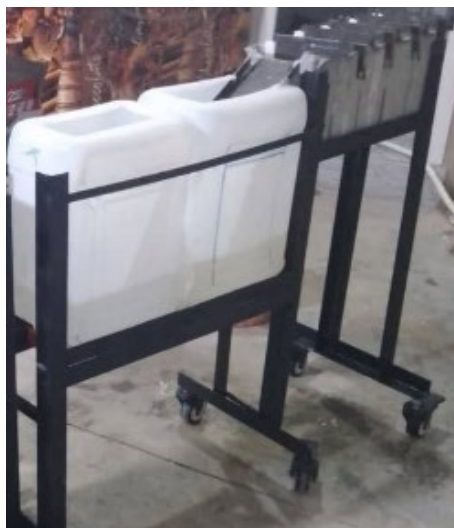
Fig. 5. Electrocoagulation treatment prototype using SVPS configuration
