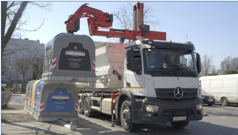
Fig. 3. Emptying containers in the PRESKO system [9]
