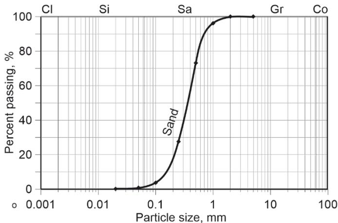
Fig. 1 Fine aggregate particle size distribution:
