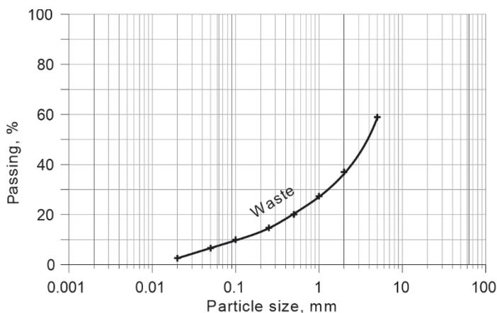
Fig. 2. Waste particle size distribution curve
