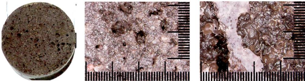
Fig. 3. Surface structure of the S-TO(6)+A sample
