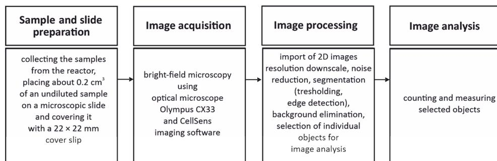
Fig. 1. Schematic representation of image acquisition and processing
