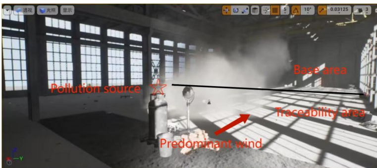
Fig. 13. Construction of 3D indoor air pollutant diffusion concentration field in UE4 environment
