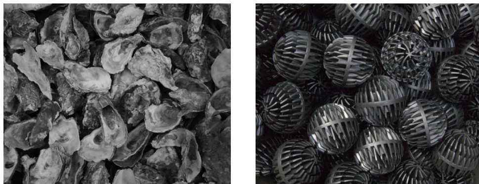
Fig. 2. Filter media: oyster shells (left), and bio-balls (right)
