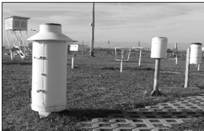
Fig. 1. Rain gauges in the IMGW meteorological station in Legnica (from left): a float and tipping bucket SEBA type, pluviographs and Hellmann's rain gauge (photo by J. Jadach)
