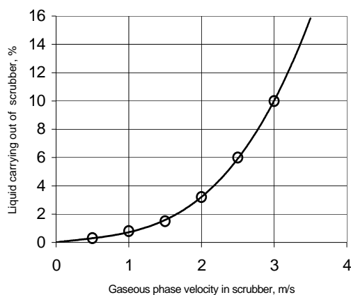
Fig. 3. Influence of gaseous phase velocity on liquid removed from scrubber
